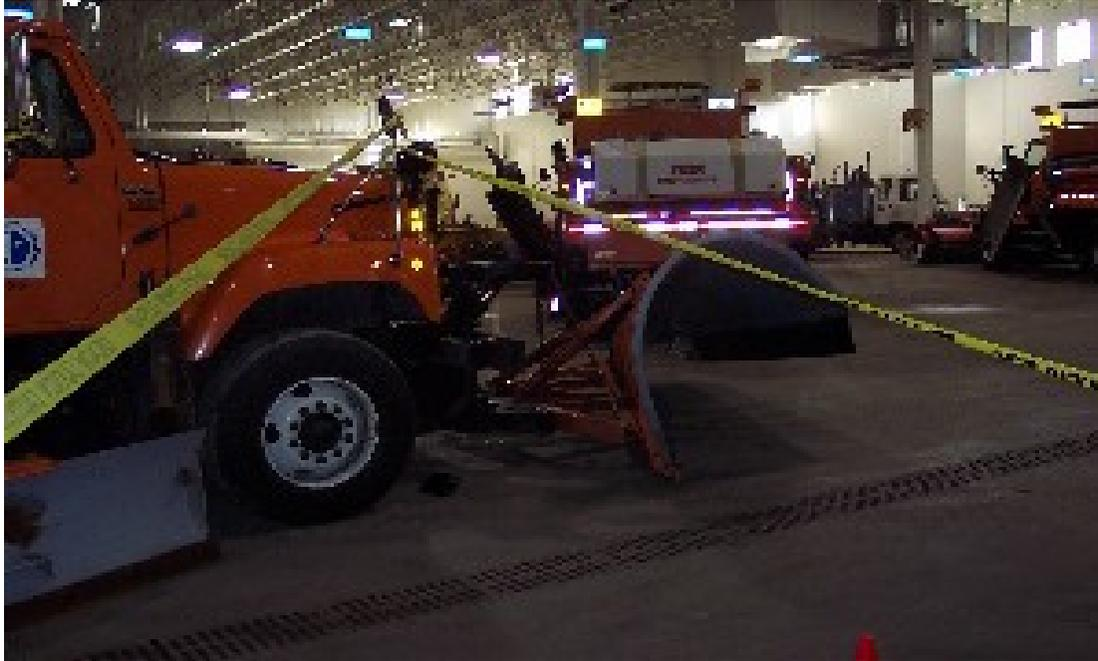
The tape at the left of the picture shows the edge of the field of vision provided by the 8-inch convex and the tape at the right shows the edge of the field of vision provided by the BDS mirror. Clearly, with the convex mirror a blind spot still exists, which we measured at 8-feet wide at a distance of 10-feet out from the center of the front axle. As the photo shows this blind spot was eliminated by the use of the BDS mirror.
