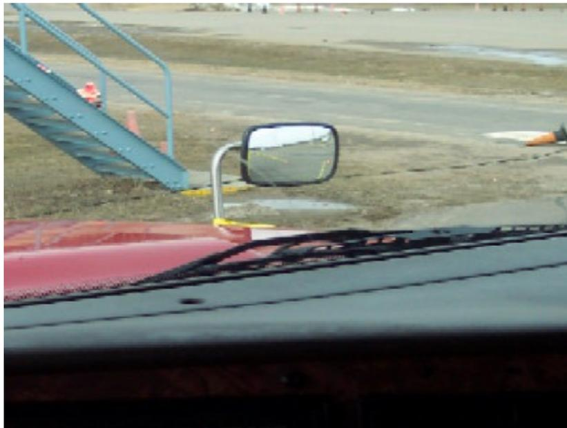
We then had the operator sit in the seat and we marked the edges of the field of vision provided by all the mirrors on the truck. We had four other drivers look into the mirrors to aid us in reaching the conclusion that we had an accurate portrayal of what could be seen in the mirrors. We placed tapes to mark the areas. We attach a photo illustrative of the taped fields of vision.
