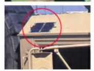
The solar panels of two 24-Volt Solargizers mounted on an Oshkosh 10-ton truck.
