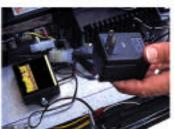
A RediPulse 6-12 installed on a motorcycle to help prevent the loss of battery power while the cycle is stored indoors.
