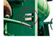
The solar panel of an Industrial 12-Volt Solargizer mounted on the side of a cotton picker.
