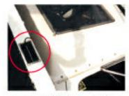
Industrial 12-Volt Solargizer units being used to prevent the loss of battery power on a fleet of de-icers at a major airport.
