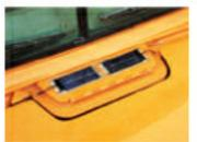
The solar panels of two Industrial 12-Volt Solargizers installed on a concrete truck.
