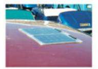
The solar panels of two 24-Volt Solargizer systems mounted on top of a neighborhood electric car.
