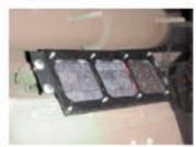
An M88 Tank Recovery Vehicle with three 24-Volt Solargizer solar panels mounted on the side.
