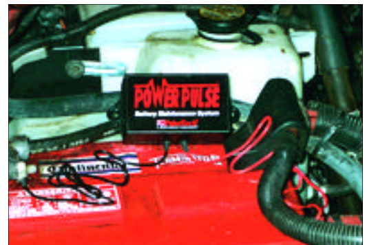
(Top) The East Texas Medical Center EMS department was suffering from dead batteries because of parasitic drain on ambulances sitting unused. Since installing the 12-Volt PowerPulse system (bottom) 17 months ago, they have had very few problems.
