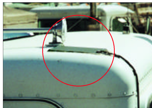
(Top) One of 500 concrete trucks used by LMC. (Bottom) The solar panel of a 5-Watt Solargizer Solar Charger mounted on the roof of the cab.
