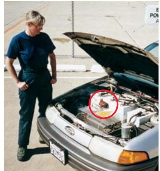
Photo: Clare Bell, electric vehicle technician/specialist for Green Motorworks and the editor of Current EEvents, stands next to an electric-powered Ford Escort using a PowerPulse to improve battery performance. (Bottom) A 48-volt PowerPulse system installed on the Escort batteries.
