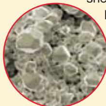
(Left) A battery plate covered in heavy sulfation buildup which reduces the battery's ability to accept, store and release energy. (Right) ReNew-It Pulse Technology™ cleans these lead-sulfate deposits off the plates and converts them to active electrolyte. This process exposes the active material on the battery plates which means batteries are stronger so you get up to three times longer life and maximum performance.
