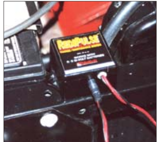
(Top, middle) J.D. Ryan, co-host of the Russ Martin Show in Dallas, Texas, standing on his boat. (Bottom) One of two RediPulse 6-12 Charge/Maintenance Systems connected to the boat batteries. By keeping the batteries sulfate free, the boat started after sitting unused for five months.
