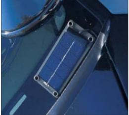
Photos: The city of Coppell, Texas installed Industrial 12-Volt Solargizers (bottom) on its entire fleet of police cruisers (top). Solargizer not only maintains peak battery efficiency, the solar panel helps offset parasitic drain due to lights, sirens, radios, etc.
